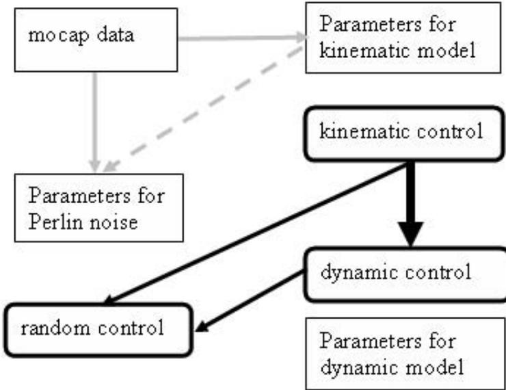
**Fig. 1.** The three procedural control paradigms, gray arrows showing off-line parameter acquisition based on information from other methods. The other arrows show the possibility for information exchange for real-time parallel tuned usage of multiple methods. The thick arrow indicates the novel method discussed we implemented.
